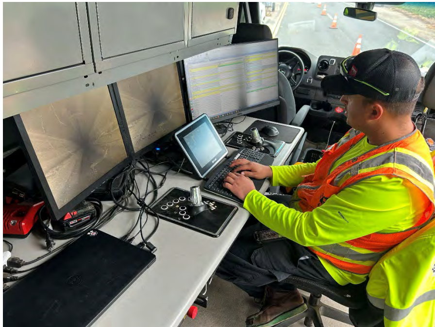
Figure 4 – Video Inspection of OH Pipeline at Rose Ave. and Walnut Dr. on November 24.
