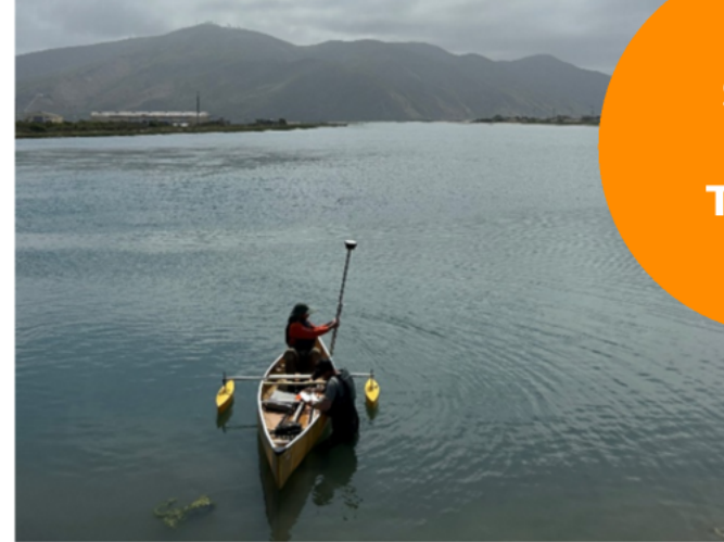
Single-beam echosounder with RTK-GPS
