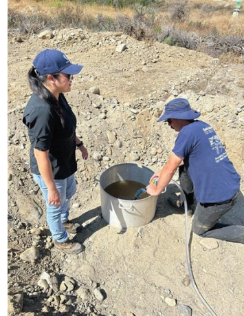
Groundwater Infiltration Testing at SFD - July 2025
