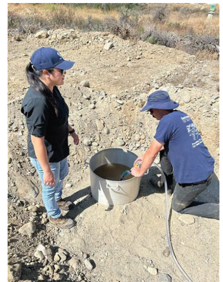
Groundwater Infiltration Testing at SFD - July 2025
